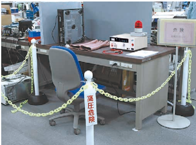
▲The picture shown above indicates the caution sign of "HI VOLTAGE DANGER" with a chain surrounding the test site.
