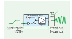
Voltage amplification rate: 13.5-times or 27-times
