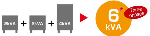
\*8kVA when used in the "Unbalanced Three-phase"
