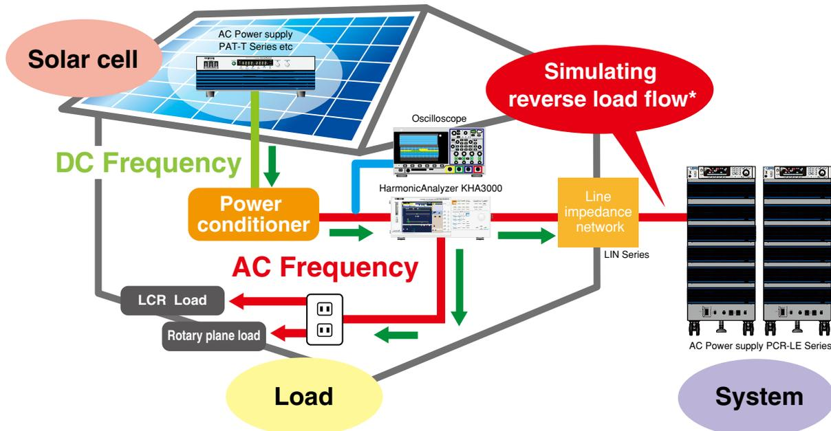
\*All the simulated reverse load flow power is consumed internally, thus, there will be no reverse load flow to the system.
