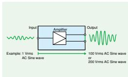
Voltage amplification rate: 100-times or 200-times
