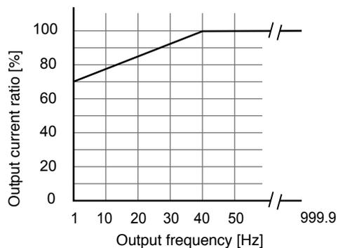
For the “Output voltage ratio versus rated output current characteristics (AC mode)” and “Load power factor versus rated output current characteristics” graphs, the rated output current is the product of the output current ratios shown in both graphs. The output current ratio shown in the “Output frequency versus rated output current characteristics” graph is given priority if it is less than the product of the output current ratios described above. (This only applies to AC mode.)
